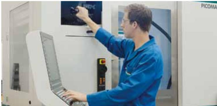
**Rapid and versatile:** Rapid retooling and efficient series production of any size down to just a single item—thanks to simultaneous loading and an automatic tool changer that can handle up to 80 tools.
