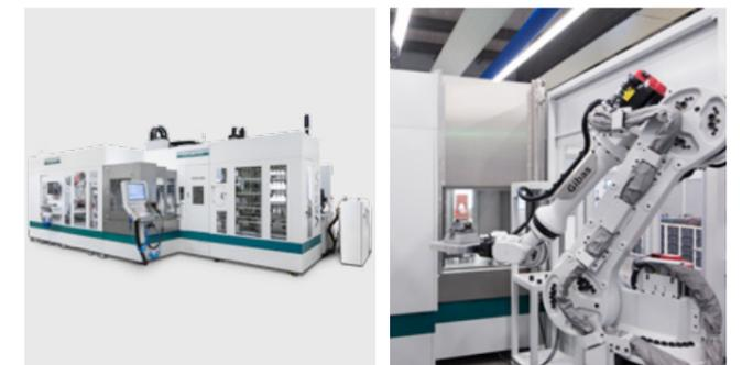
Gibas articulated-arm robot and Soflex job management system on a VERSA 825
