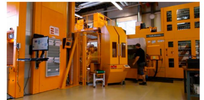
Articulated-arm robot and Goodj automation system on a VERSA 825 with rack magazine for 346 tools
