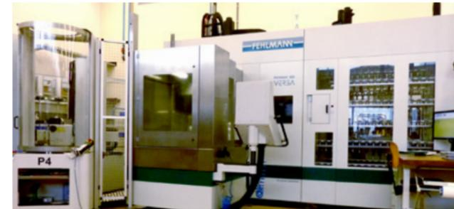
With the VERSA 825 by Fehlmann, the company managed to reach 5000 operating hours a year in two shifts, including unmanned operation.
