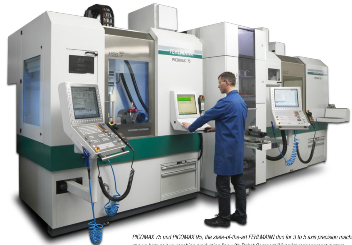
PICOMAX 75 und PICOMAX 95, the state-of-the-art FEHLMANN duo for 3 to 5 axis precision machining — shown here as two-machine production line with Robot Compact 80 pallet management system.
