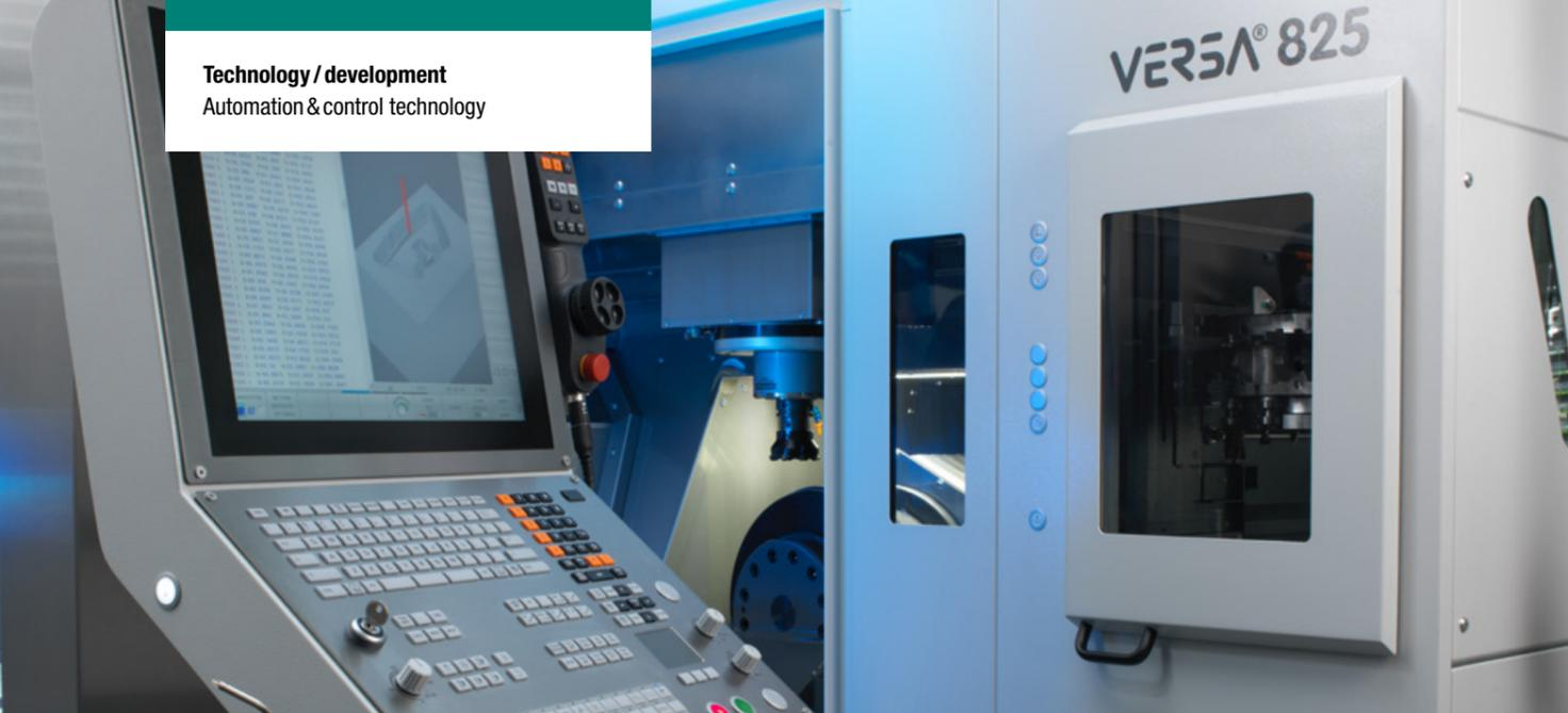
Heidenhain TNC 640 with touch screen on a FEHLMANN VERSA 825
