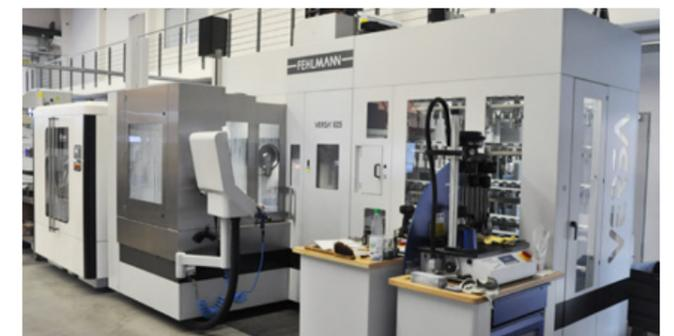
LANG ECO Compact 20 on a VERSA 825, actuated via M functions
