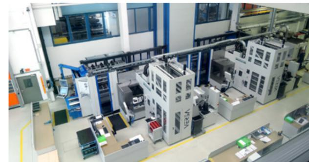
Linear automation solution consisting of two VERSA 825 with rack magazine for 346 tools each
