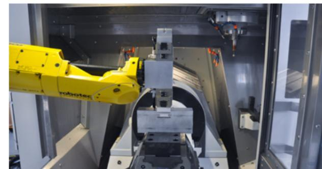
Articulated-arm robot for handling pallets and blanks on a VERSA 825
