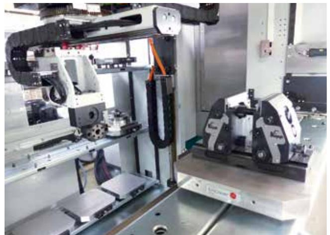
**2** The Erowa robot Leonardo carries in its standard version up to 24 UPC palettes (320 mm × 320 mm). The production unit is primarily used to manufacture cages made from case-hardening steel for roller burnishing tools (Photo: Fehlmann)
